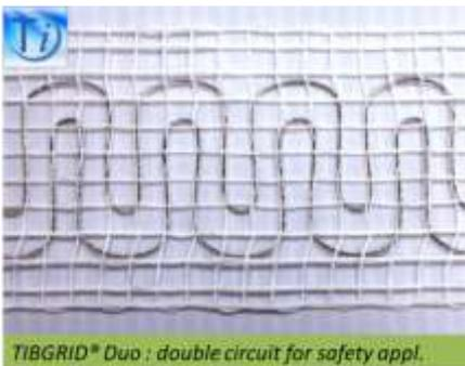
TIBTECH has developed, for some aerospace applications where safety is a major issue, a double circuit where each of the circuits are exactly covering the same heating zone. (see fig. ) They can be switched on independently practically immediately in case of damage or electrical malfunction.
